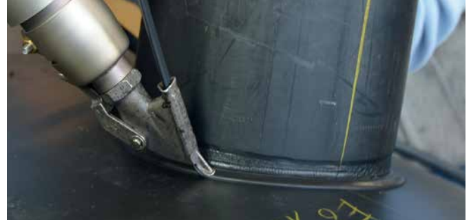
Draw welding with combination nozzle
